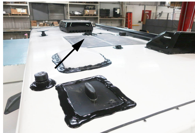
3-Port Solar Cap (Located on the roof) -Typical View
